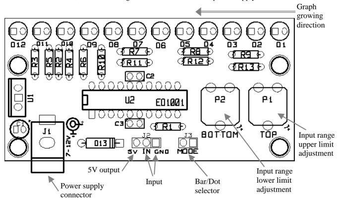
By default the module is in bar mode; to enable dot mode, insert the provided jumper into J3.
